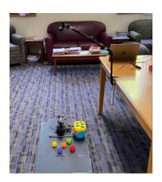
In this image to the left you can see my setup for the summer. The shape toy and robot were on a table top on the ground. Attached to the table is a webcam that overlooks the whole scene. This webcam is what took the pictures used in the computer vision discussed later.
