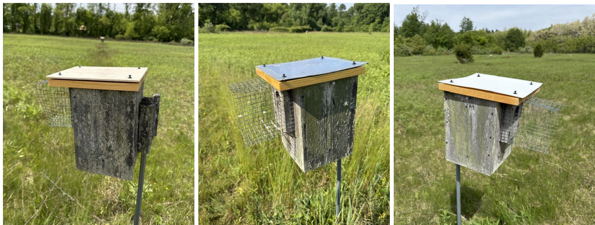
Figure 1. The three variants of second roof installed onto pre-existing nest boxes. From left to right the materials are plywood, aluminum, and plastic.
