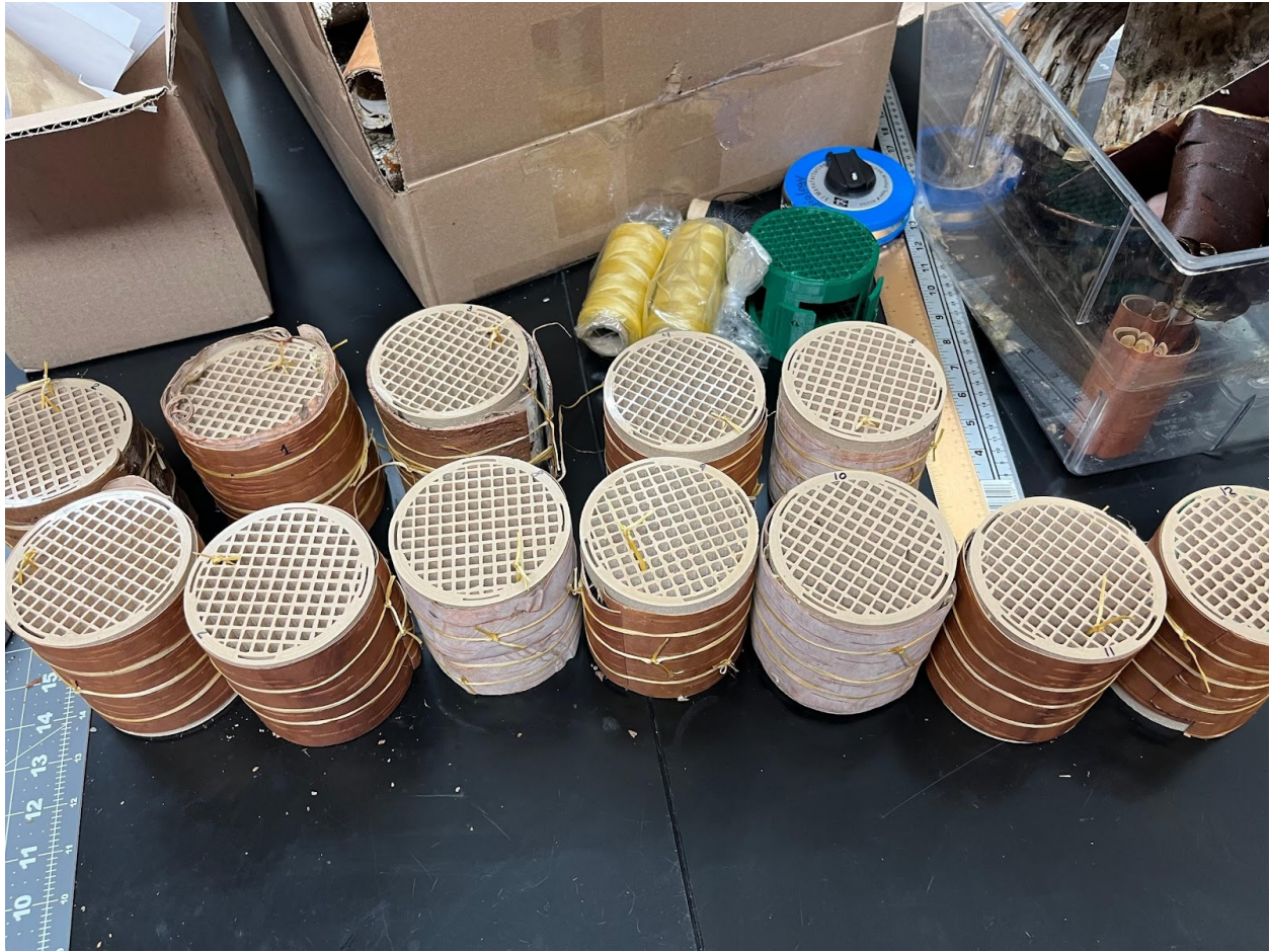
Finished 3D printed plant based macroinvertebrate collectors with birch bark wrapped around.
